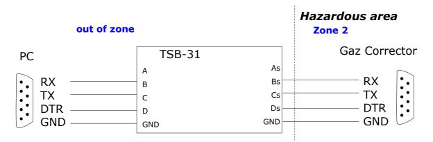
Note that RS-232 norm specifies that RS-232 voltage can be up to  $\pm$  15V. With such voltage, the protection diodes will clamp the voltage and drain a high current and possibly blowing the fuse.
